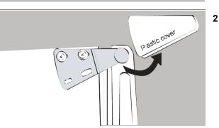
3. To install the top hinge on the left side of the appliance, secure the two screws through the hinge and into the top of the appliance. Slide the door back on to the top hinge. Ensure the door is face up. Replace the top hinge cover on the top hinge by pressing down until it clicks into position.
