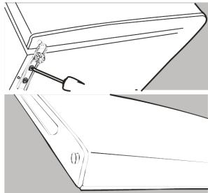
2. Remove the top hinge cover from door first. Then unscrew the two screws from top door hinge and replace on the other side.
