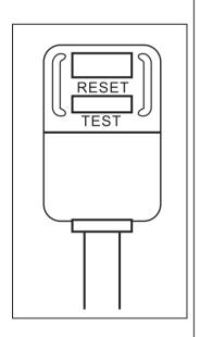
Your portable air conditioner is supplied with a Leakage-Current Detection and Interruption (LCDI) plug. This plug reduces the risk of fire due to arcing faults in the power supply cord. Please follow the instructions below to ensure that LCDI plug works properly.
