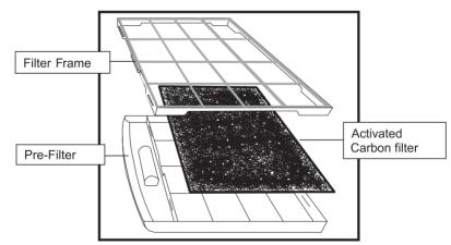
An optional  $3M^{\text{TM}}$  Filter can also be purchased to replace the activated carbon filter. The  $3M^{\text{TM}}$  Filter has an agent that helps inhibit the growth of mold and mildew on the filter. This filter is electro-statically charged for enhanced particle capture and retention.
