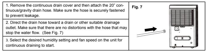
NOTE: When using continuous/gravity drainage setup, there may be some water collected in the water in the drain bucket
