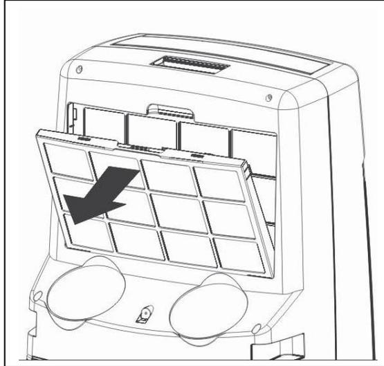
2. Remove the filter frame from the pre-filter
