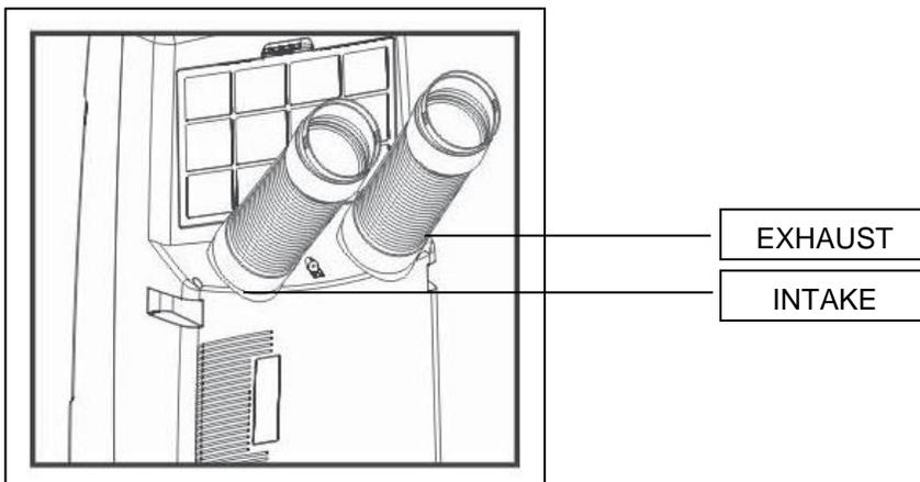
If installing the optional air intake hose in an area with poor air quality, we recommend purchasing the intake hose pre-filter accessory.
