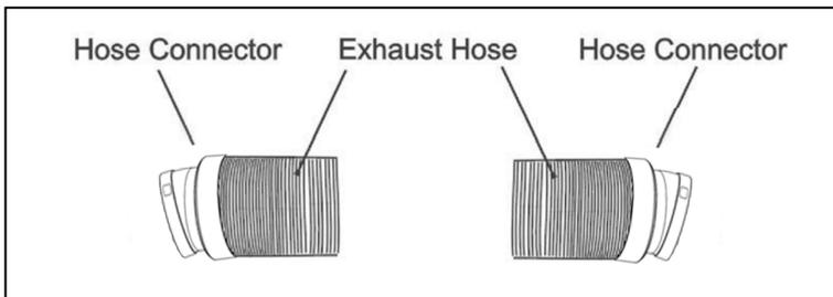
3. Align the tab cut-outs of each of the hose connectors to the tabs on the air exhaust and air intake at the rear of the unit and snap in place.
