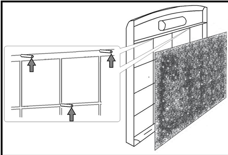
3. Once the activated carbon filter is secured, insert the assembled filter frame into the unit.
