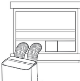
Hung Window Installation
