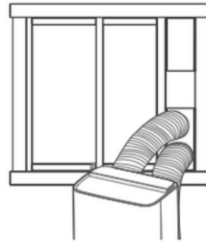
Sliding Window Installation
