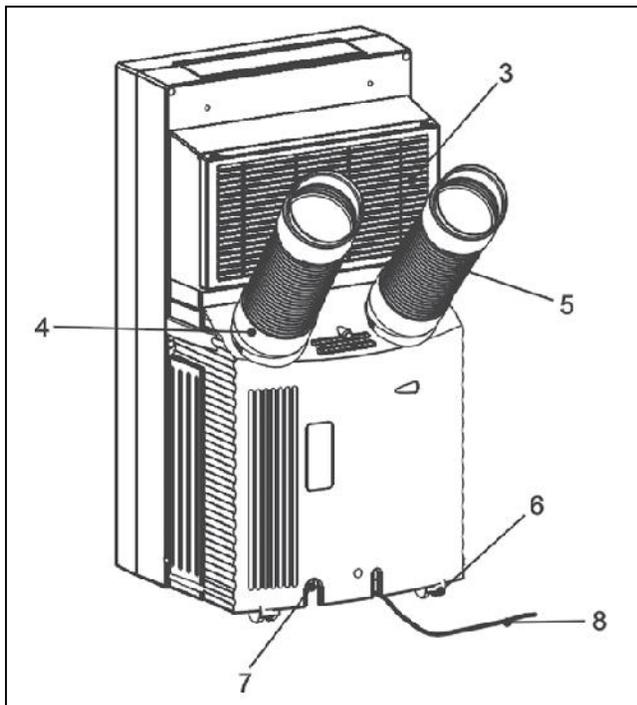
3. Evaporator air intake / air filter
