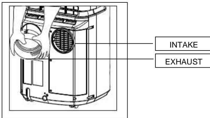
5. Only extend the exhaust hoses to the necessary length. We do not recommend extending the exhaust hose more than 9' long. Additional 4' exhaust hose sold separately.
