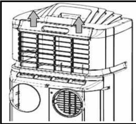
2. Place the activated carbon filter on the pre-filter frame by inserting it through the three pins.
